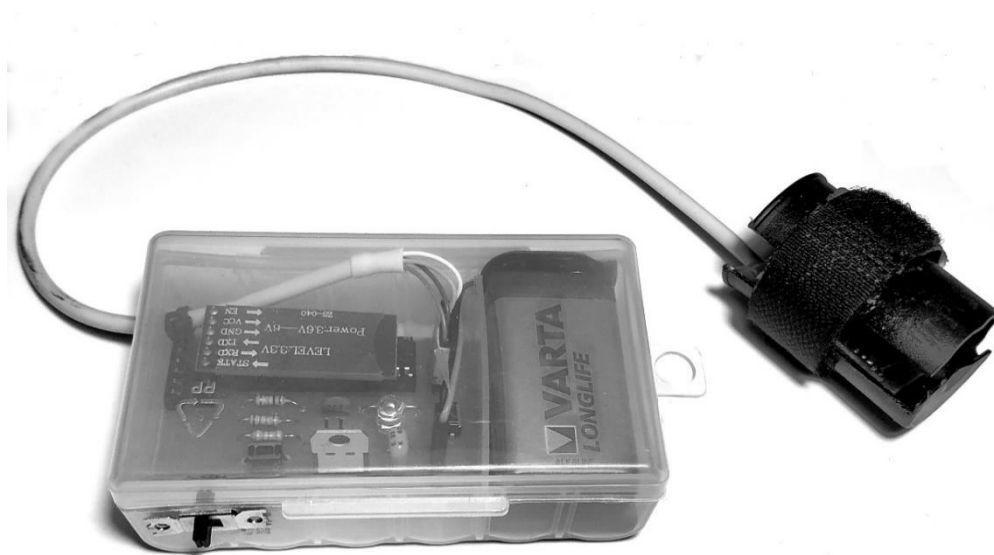
Figure 2. The wireless computer communication system, via Bluetooth, which was built in the Department of Physics of UoI.
